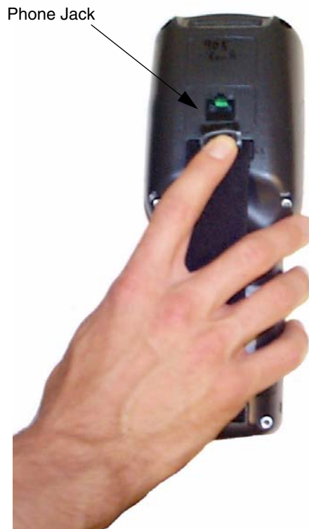
Phone Jack on rear of Dolphin 7400
